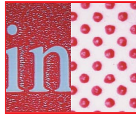
Cushion-Mount™ Plus Soft Combination Printing Tape provides soft support that helps improve tone reproduction when process and halftone images predominate. e.g. 1920M Tape
