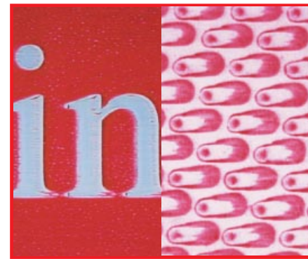
Cushion-Mount™ Solid Printing Tape uses a foam carrier instead of vinyl to help reduce cylinder bounce and deliver results similar to Flexomount™ Tape. e.g. 939 Tape
